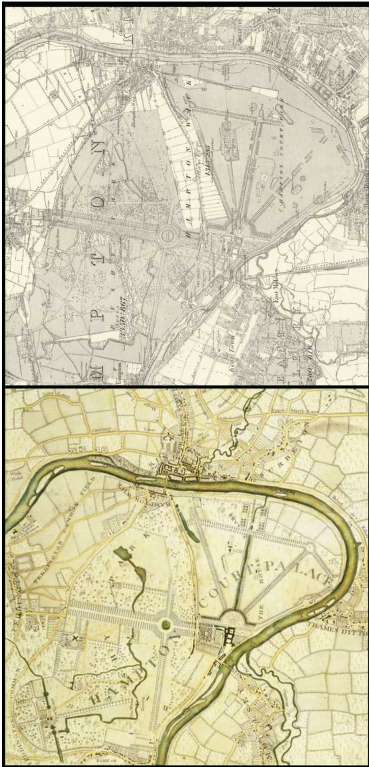
Two maps of The Royal Parks: Jean Rocque 1730 (l) and Ordnance Survey 1868 (r). The use of theodolites to create the later map account for its greater spatial accuracy but the details correspond to a remarkable degree. Note the presence of the Royal horse paddocks in the later map.
